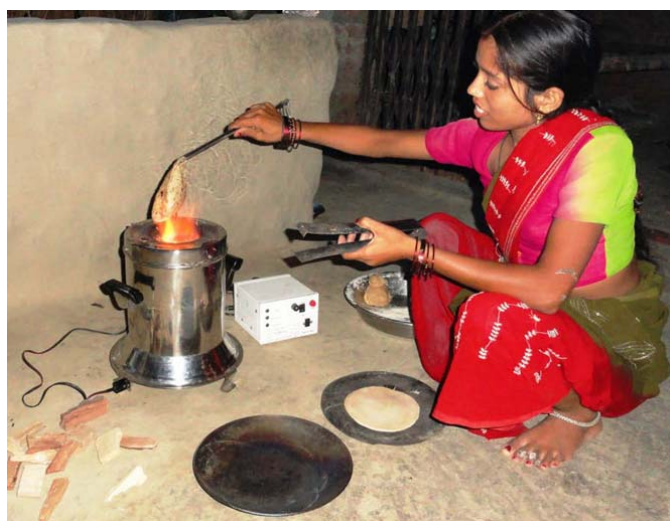
Forced air stove with electrically powered fans and rechargeable batteries for use with photovoltaic cells. Source: TERI (India), www.rbsgroup.in
