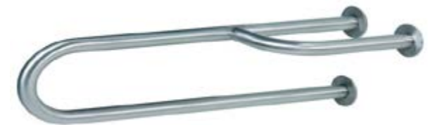
Stainless steel tube can easily be bent to the desired geometry and welds can be polished to a point where they become indistinguishable from the original surface. Photo: Mediclinics, Barcelona, Spain
