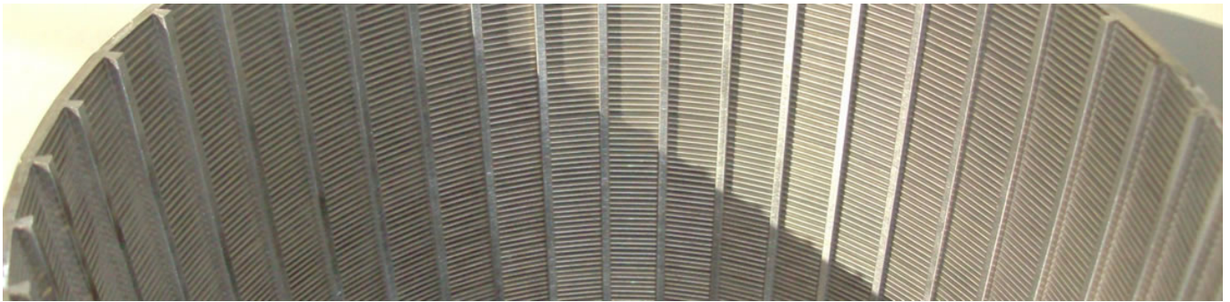
Water intake filter made from stainless steel wedge wire.
